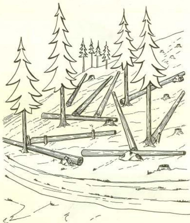
Fig. 46. Securing logs on steep terrain to prevent them from rolling or sliding downhill.
