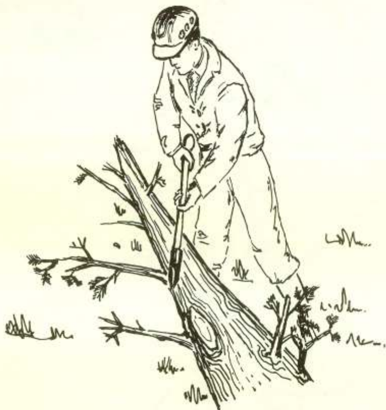
Fig. 49. Correct position for branching. The safest practice is to stand on the side of the tree opposite the branch that is cut.
